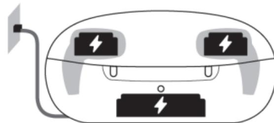
As long as the charger is being charged by an external power source, charger LED shows the charging status of the integrated battery and the LEDs for the hearing aids show the status of the hearing aids.
