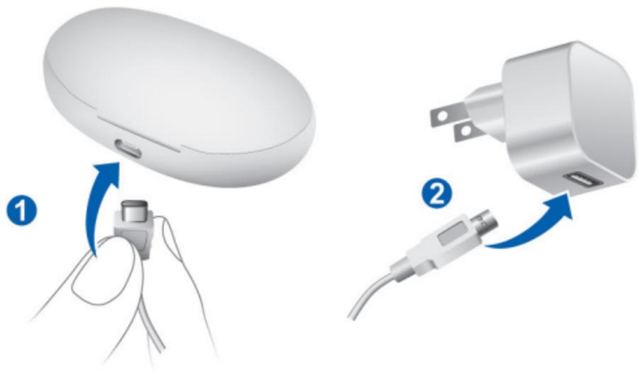
The internal battery starts charging. When hearing aids are inserted, they start charging as well. The charging status of the charger is shown permanently.
