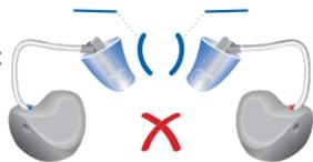
Hold the receiver cable at the bend closer to the ear piece.
