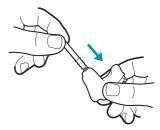
2. Pull the application stick straight out to remove the used wax guard. Do not twist.
