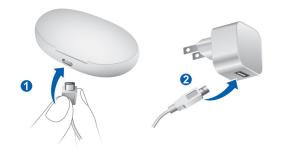
The internal battery starts charging. When hearing aids are inserted, they start charging as well. The charging status of the charger is shown permanently.
